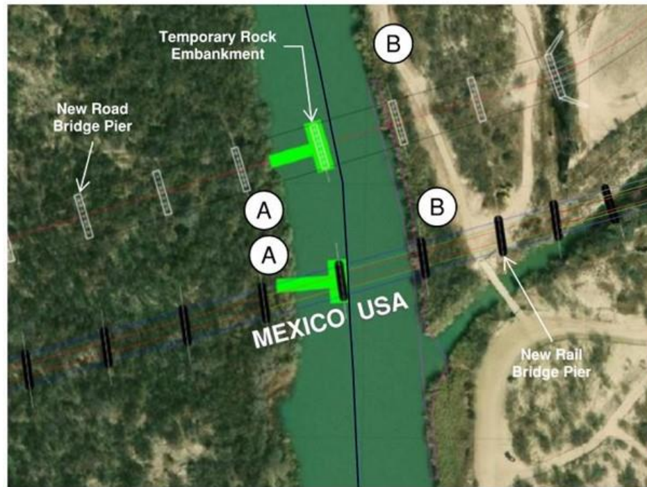
Figure 7. New Rail Bridge (Northern Rail Alternative) and New Road Bridge Construction
